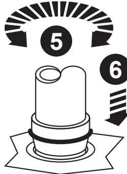
⚠ **CAUTION** - Rubber sealing ring should sit tight against the top edge of the floor receptacle.
