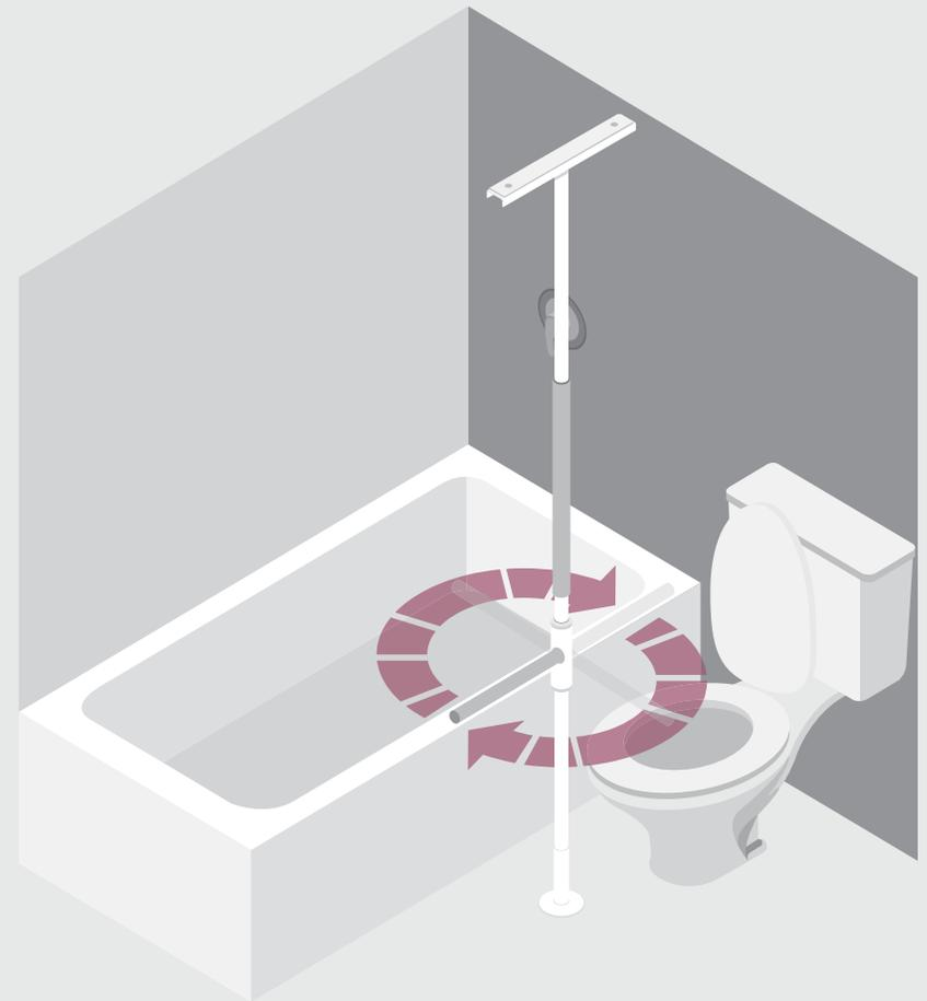
The SuperBar is designed for complete bathtub and shower support that in some cases, replace the need for multiple grab bars. The horizontal rail moves and locks every 45 degrees, to create a comfortable and ergonomic weight-bearing support.
