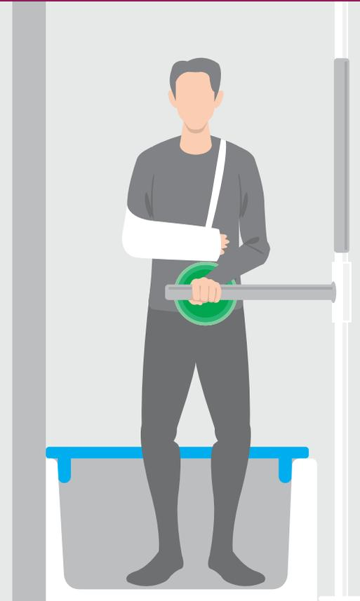
If the client has an injury that hinders the side closest to the vertical SuperPole, the SuperBar can be located in front of the client. This position maximizes the clients' abilities, and eliminates dangerous body twisting.
